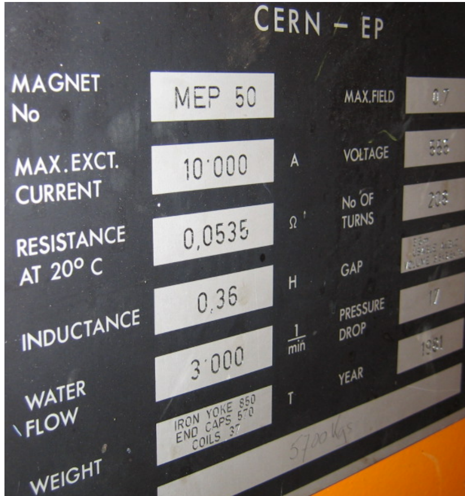
Figure 5.9: Specs of the UA1/NOMAD dipole magnetic [18].
